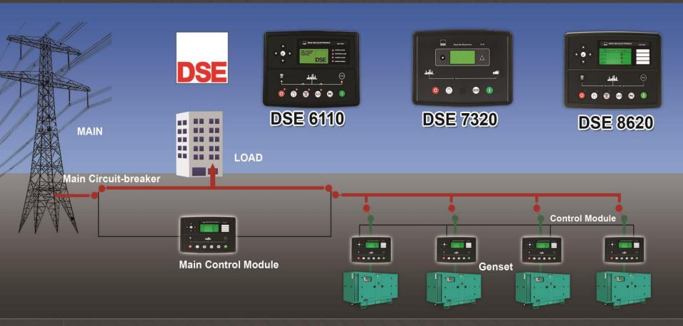
Monitoring speed, frequency, voltage, current, oil pressure, coolant temperature and fuel level, the modules will display warnings, shutdown and engine status information on the back-lit LCD screen and illuminated LED.
